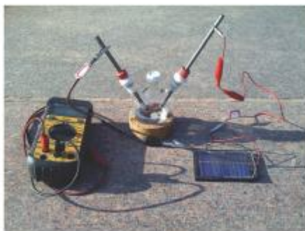
Fig. 1 An electrochemical reaction setup with a simple 6 V photovoltaic power supply is shown. The ammeter is spliced into the line so that the current passed through the flask can be monitored.
