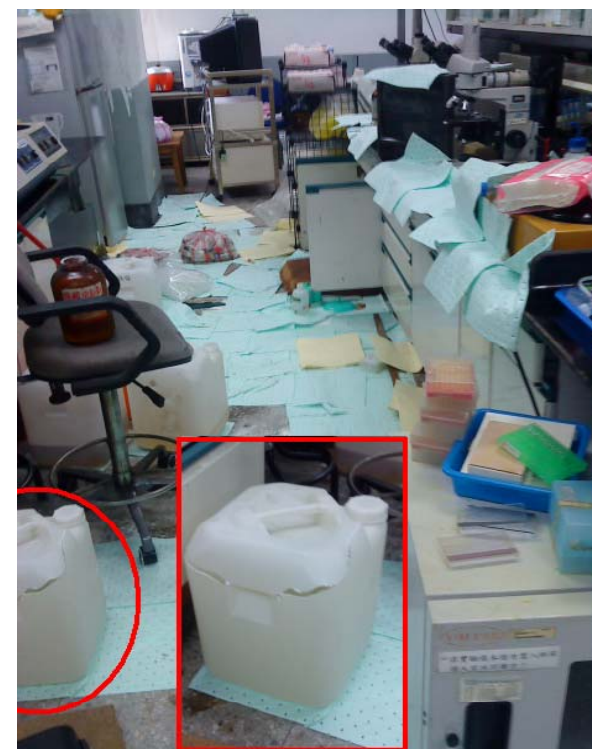
Mixing organic waste with waste acids causes explosion
