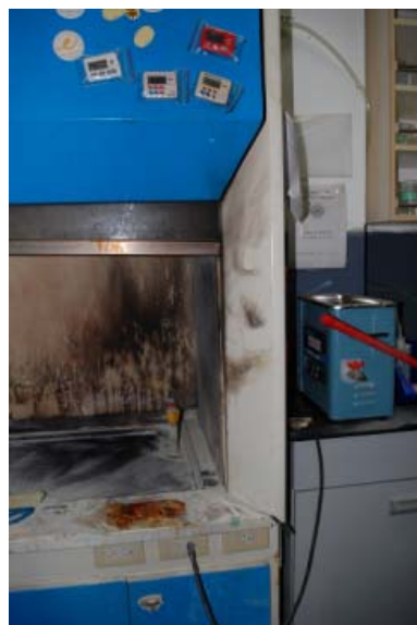
Mixing KMnO 4 /H 2 SO 4 /toluene causes fire
