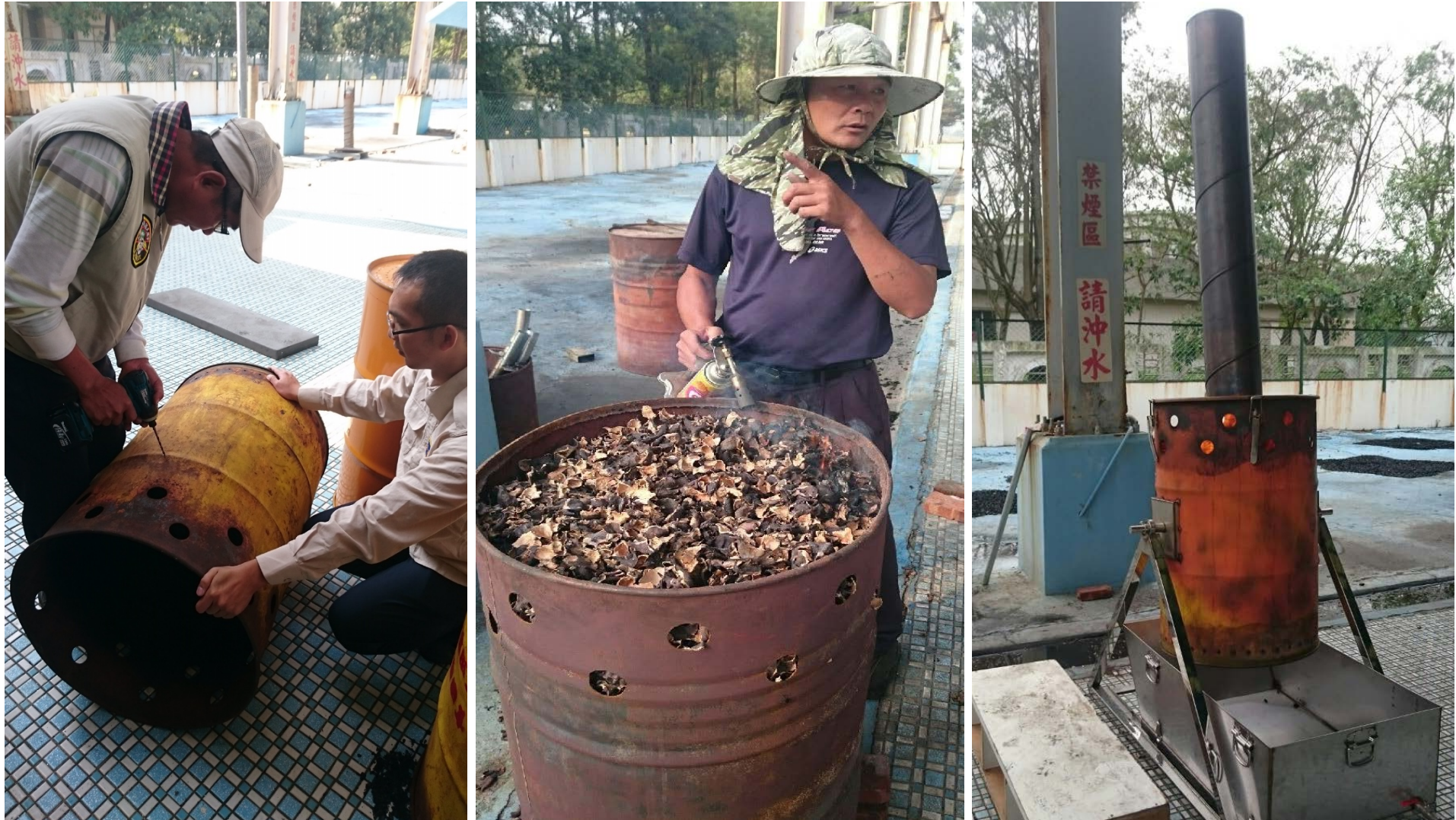
Carbonization furnace first set up in November, 2015
